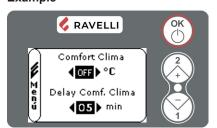
To activate the function, set the COMFORT CLIMA value different from OFF using buttons 1 and 2. Confirm with OK.
