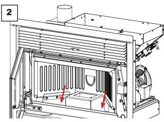
Vacuum the residues present in the ash compartment with a suitable ash vacuum cleaner, making sure that the ashes are completely extinguished.
