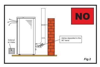
It is prohibited to install a 90° bend for the initial segment, since the ashes would quickly obstruct smoke passage, causing draught problems in the appliance. (See Fig. 2)
