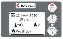
The modulation phase is activated, as the room set temperature has been reached. If the temperature is maintained for the set "DELAY COMFORT CLIMA" time, the stove switches off.
