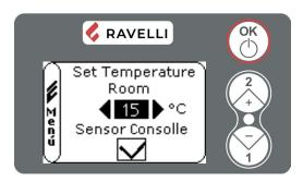
Set the desired temperature with keys 1 and 2. The selectable values are: EST, from 7 °C to 40 °C (or from 44 °F to 104 °F), MAN. The EST value must be selected if you want to use the external thermostat and MAN when you want to make the stove work at constant power.
