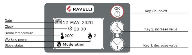
Key "OK": in the Home screen, long press to turn the appliance on / off or reset the alarms; short press to enter the menu
